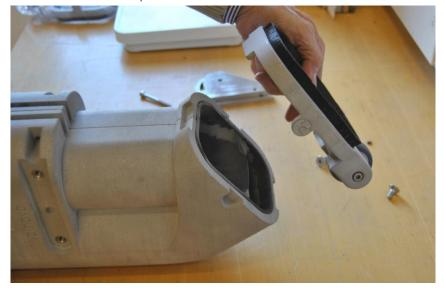
5. Open the three screws in the front of the housing.
