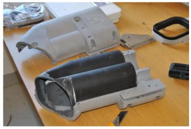
8. The wear rubber parts of the PiWalk housing consist of three parts. The two parts shown below should be inserted first.
