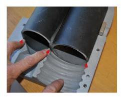
9. Insert the nozzle into the housing. Press the housing parts together.
