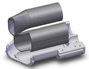
It is important that the glued connection of the wear parts is aligned with the edge of the PiWalk housing.
