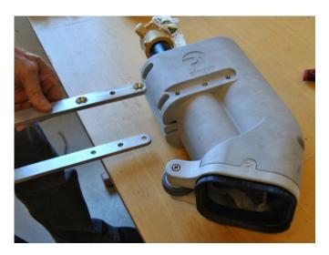
3. Remove the steel parts of the handle fixture by opening the two screws, as shown below.
