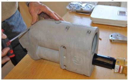
6. Use a sharp knife to cut loose the rubber from the housing. Open the housing.
