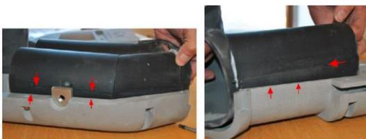
Align glued connection of the “wear part assembly” (1) with the upper rim of the housing (11) as indicated by the arrows
