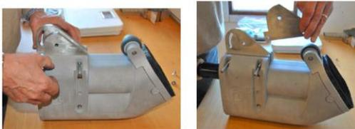
Detach “handle assembly” (9) from main housing (10, 11) by removing the two screws (4)
