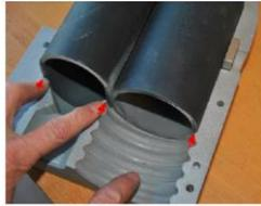
Align upper end of “wear rubber assembly” as indicated on the left
