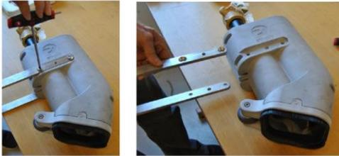
Detach “wheel suspension assembly” (7) from main housing (10, 11) by removing the four screws (8) as shown on the left
